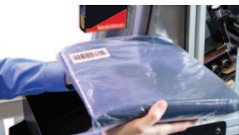
Mailing labels are automatically printed and applied, and the bag sealed as it exits the bagger
