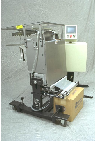
Operated horizontally, the wide bagger is ideal for difficult hand-load applications
