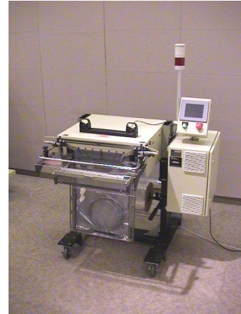
Operated vertically, the wide bagger easily handles loads up to 16 inches wide
