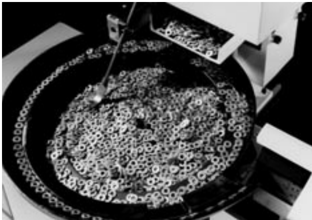
Continuously high speed rates are achieved through the combined action of a unique vibratory bowl and interrupting accumulator.
