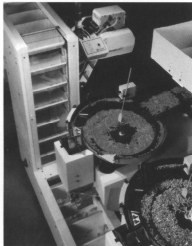
Mixed products are counted by any number of vibratory Accu-Count® counters, dispensed into Kit-Veyor buckets, and batched into bags, in custom-indexed profiles, for continuous or intermittent conveyance and packaging to suit particular kit-making requirements.
