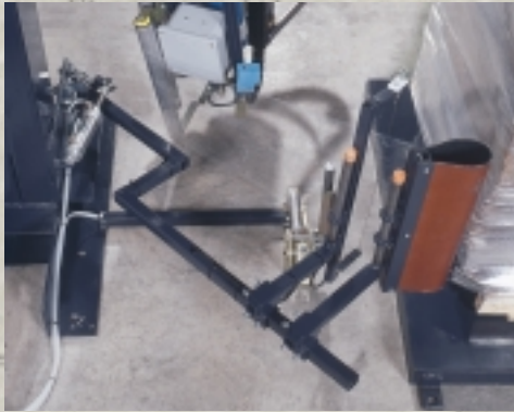
At the end of the wrapping cycle, Orion's innovative asymmetrical film clamp grips the film web while the impulsed wire cuts the film. Then the load seeking brush smooths and secures the film tail to the side of the load. The result is a film tail that stays in place and an attractive load to present to your customer with no unsightly film tails.
