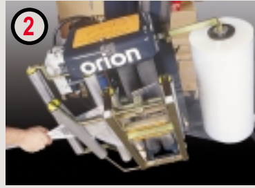
2 ...next, open the hinged roller frame and pull the film web through...
