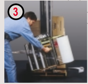
3 ...finally, latch the roller frame closed, activate power and pull film through. That's all there is to it!
