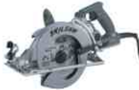
SKIL 7-1/4" WORM DRIVE SAW 13 amp 4,400 RPM 16 pounds
